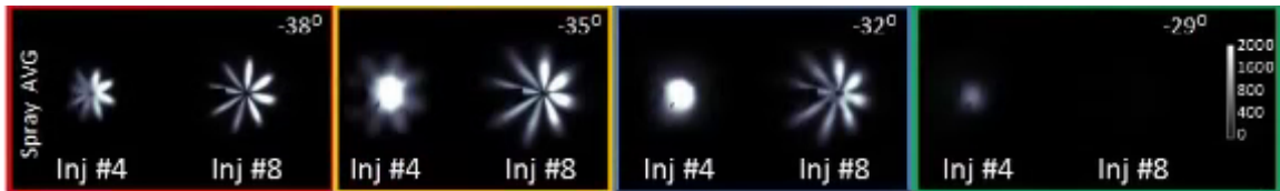
Figure 3.9: Comparison of EDM (Inj #8) and laser drilled (Inj #4) nozzle sprays at various crank angles, reproduced from [120].
