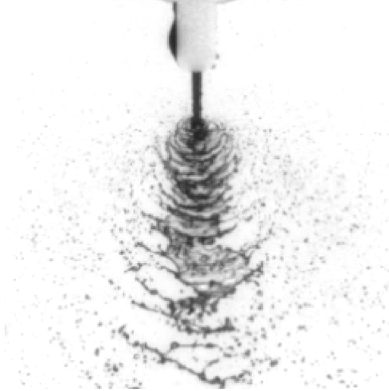
Figure 5.1: Visual light image of the impinging jet spray used in the experiments, reproduced from [50]. Re = 10,300 .
